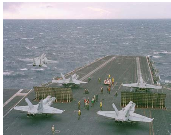
Figure 16. Catapults and jet blast deflectors.
