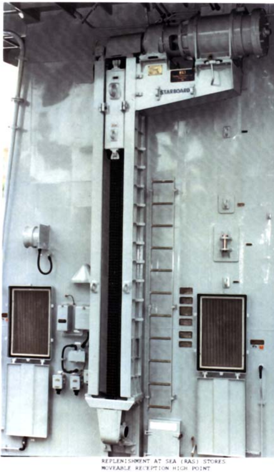
Figure 17. Typical transfer high point mechanism.
