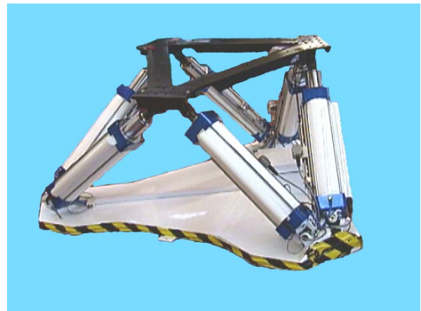
Figure 15. Six-axis Stewart Platform
